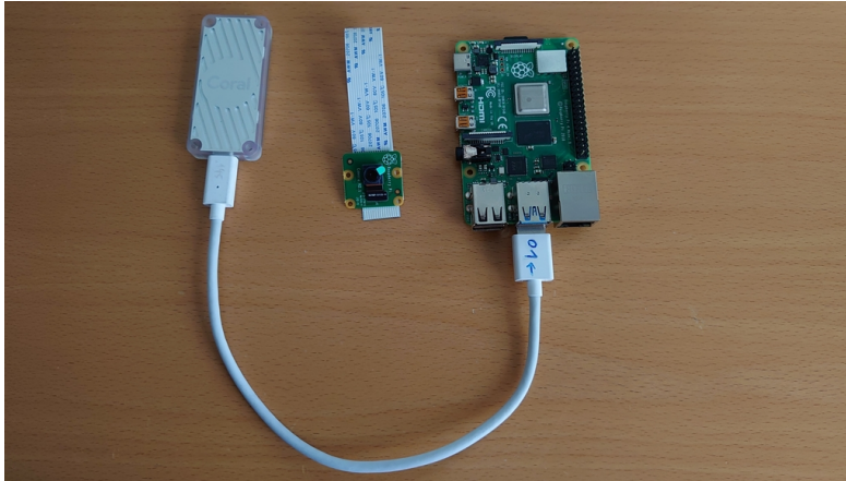
Figure 2.5: Edge hardware including Raspberry Pi, Edge TPU and camera module.
