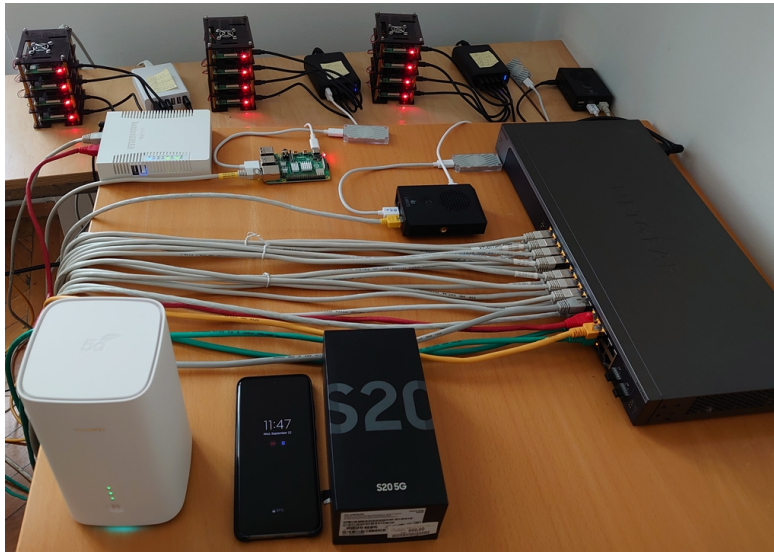
Figure 2.6: A testbed infrastructure for evaluation of edge data analytics approaches.
